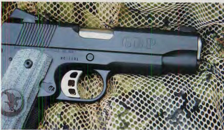
(top) Among the few parts not finished in matte black PermaKote are the GRP II's stainless steel barrel and bushing and its alloy match trigger. Note the slide stop pin machined even with the frame. (middle) On the GRP II's G10 grips is laser engraved the Nighthawk logo and the sights are genuine Novak Extreme Duty Adjustable Night Sights. (bottom) No full-length guide rod here. The GRP II is a pistol meant for serious defensive use and easy field-stripping.
