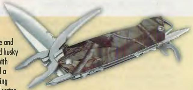
The pliers have integrated wire-cutters (10 gauge). The 3" drop-point blade, of 420HC stainless, is partially serrated, has grip ridges for blade control and a thumb stud for easy opening. Easy-slide screwdrivers are a #2 Phillips and a 3/16" square bar. The durable thermoplastic handle has a steel frame, ergonomically shaped for comfort. It comes with an easy-to-carry sheath. It is 7-1/4" open, 4-1/4" closed. It weighs 5.6 oz.
